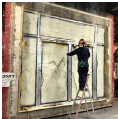
For the duration of the test nothing may ignite on the protected side. The testing officer makes sure of this by holding a cotton pad in critical areas.
